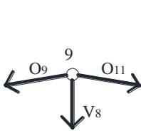
$$\sum V_i = 0 \rightarrow V_8 + \sin\alpha(O_9 + O_{11}) = 0$$
