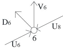
$$\sum V_i = 0 \rightarrow \cos 45 D_6 + V_6 + \sin \beta U_6 - \sin \beta U_8 = 0 \\ \rightarrow V_6 = -31,26 \text{ kN}$$
